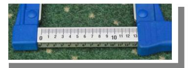
Graduation on three sides of the beam. New design of scale with resolution of 0,5 cm.
