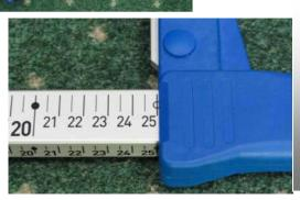
The shape of fixed handle enables to easily slip the caliper under the lying logs in order to make measurement.
